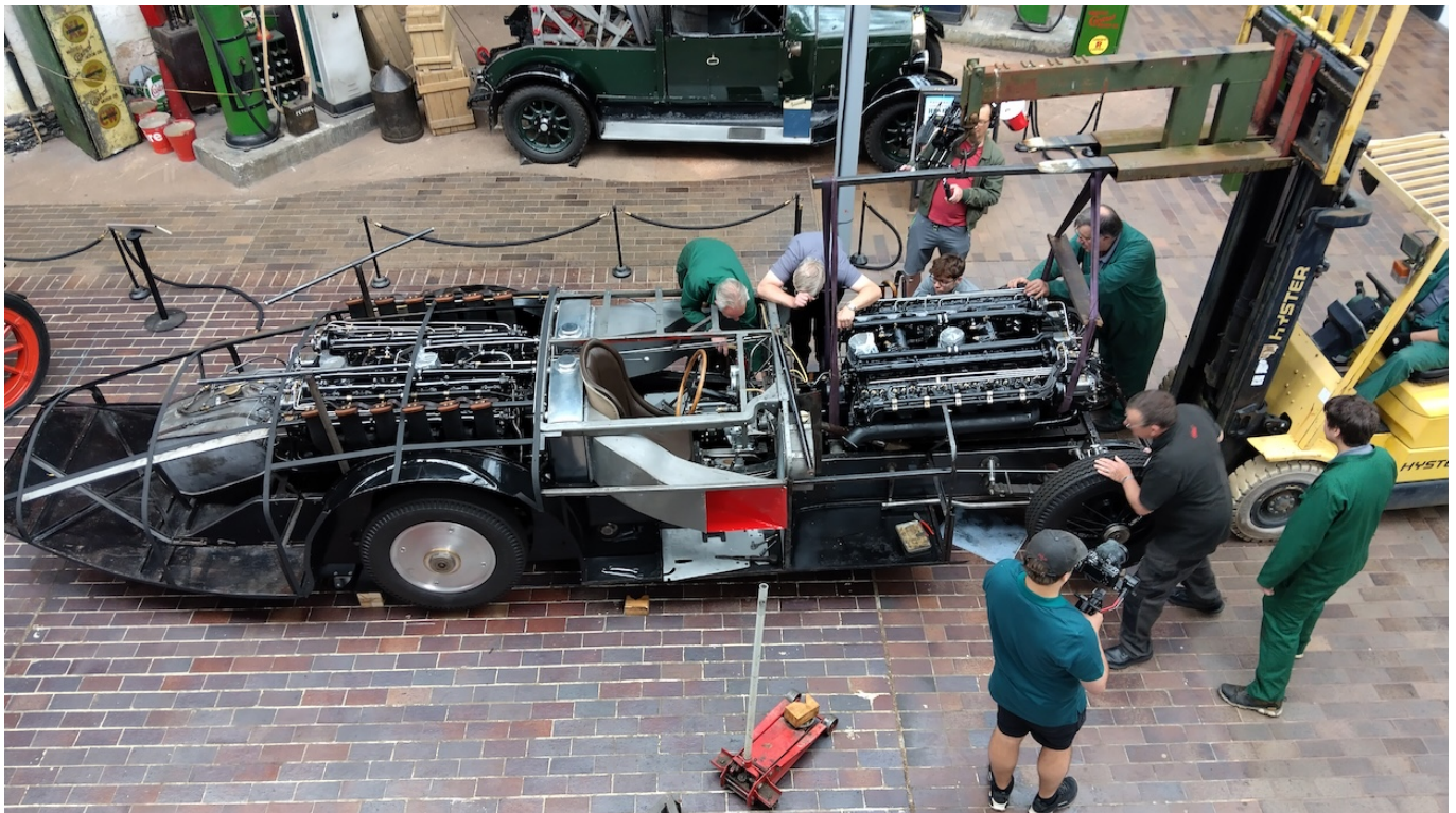
Lowering restored second engine into Sunbeam 1000hp chassis in the National Motor Museum.
