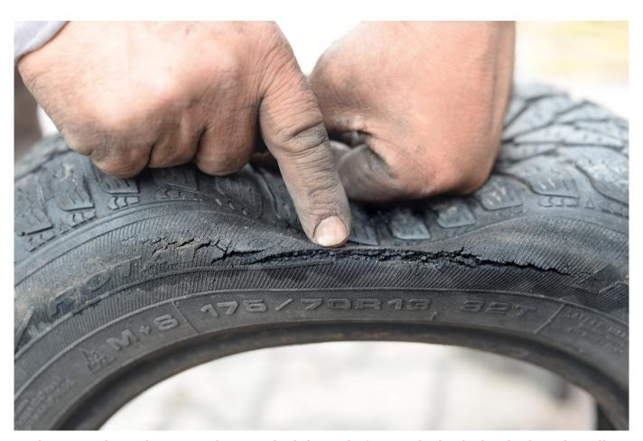
This tyre (above) has more than reached the end of its road; check closely the side walls and treads for early signs of such deterioration.
