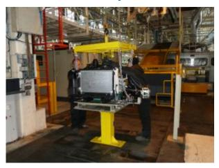
With the radiator and cooling system pipes added, the whole engine/front end assembly is cradled to the section of the line where the body shell is arriving.
