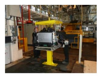
With the radiator and cooling system pipes added, the whole engine/front end assembly is cradled to the section of the line where the body shell is arriving.
