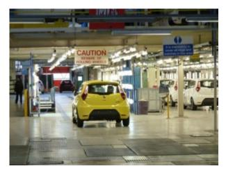
The completed cars are rolled along towards the test areas by means of a 'moving floor' system.
