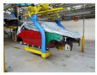
When the part-completed body shells arrive from China at the Longbridge factory, they look like this (MG3 shown here), awaiting front end components.
