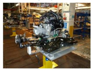
When the front sub-frame, steering rack, hubs, driveshafts and brake discs/calipers are added, the assembly looks like this.
