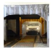
Here a new MG3 is seen as it is about to emerge from the 'Storm Test' chamber, in which each completed car is sprayed with water at high pressure.
