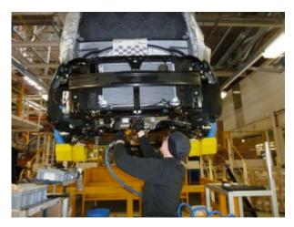
The engine/transmission/steering/front subframe assembly is raised into position from below, and bolted in (Lisa Ponter working here; please see text).
