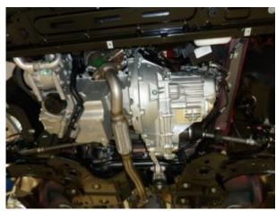
This is the engine/transmission assembly viewed from below, shown now with the exhaust system attached.
