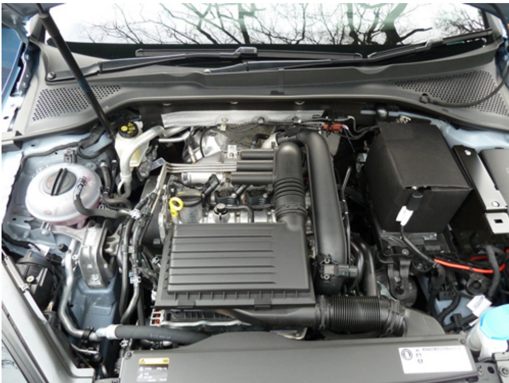
There is rather more room around the advanced 1.4 litre petrol engines than the 1.6 litre
