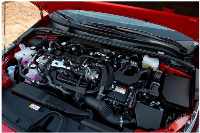
The Toyota self-charging hybrid system allows the vehicle to run on power from the engine and electric motor and electric power only as often as possible. On a light throttle the electric motor will cut in and the engine turn off and this is indicated with a green EV icon light. The EV mode can also be selected to run the car on electric power only under certain circumstances but this mode only offers around 2-3 miles before the engine seamlessly
