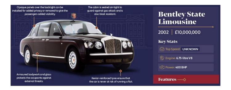
The Bentley State Limousine comes equipped with security features that one would expect the royal family to enjoy. Armoured bodywork and glass protect the occupants inside the cabin of the car from external threats, while internally, the car is completely air-tight to guard against potential gas attacks. The car also comes equipped with a blast-resistant chassis and Kevlar-reinforced tyres.
