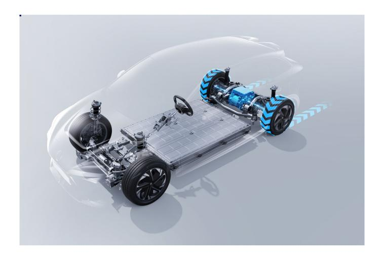
In turn this will derive its electrical energy from a choice of two battery packs (in a new battery structure that has a slimmed down height of 110mm or 4.33 in) starting with an entry level 51 kWh lithium iron battery that delivers 170 PS (125 kW) of power and promises a combined 218 mile (350 km) range, which is, perhaps, a little disappointing these days.
