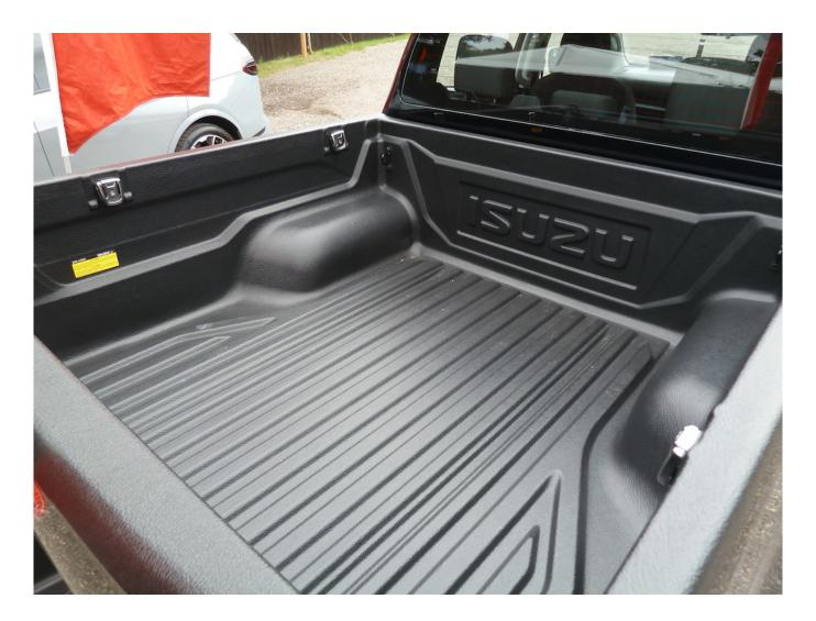
Extras fitted to the test D-Max included fitting accessories, such as tailgate assist, rubber floor trays, a tow bar, 13-pin electrics, and an over-rail load-bed liner.
