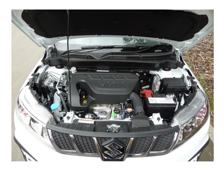
The compact 16 valve, four cylinder engine has a capacity of just 1373cc, but delivers a bighearted 140 PS at 5,500 rpm, plus 220 Nm (162 lb.ft) of torque through a wide rev band from 1,500 to 4,000 rpm.
