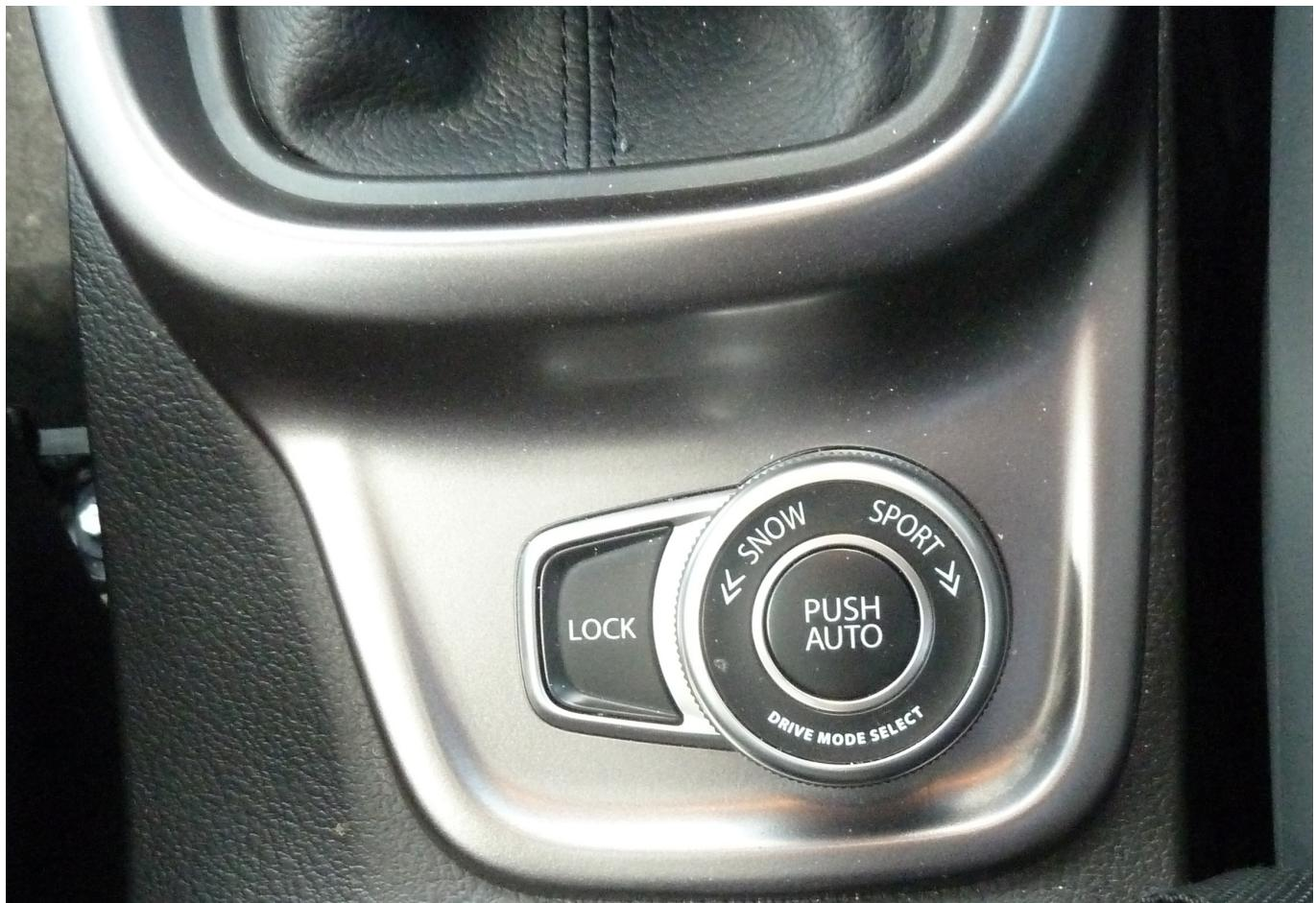
Optionally fitted to the Vitara and S-Cross in both manual and automatic versions, this electronically-activated system is driver-operated by a rotary 'push and turn' control with 'Auto', 'Sport', 'Snow' and 'Lock' settings.
