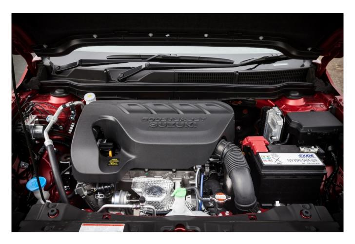
It is in the areas of engine, transmission and ALLGRIP that the S-Cross really scores, plus being the right 'middle ground' size in a competitive market. The 1.4-litre, four-cylinder Boosterjet petrol engine uses direct injection coupled with a small capacity, high torque turbocharger with the Boosterjet function controlling the wastegate valve, reducing boost pressure losses and turbo-lag. The 140 hp output is impressive enough but the secret to this
