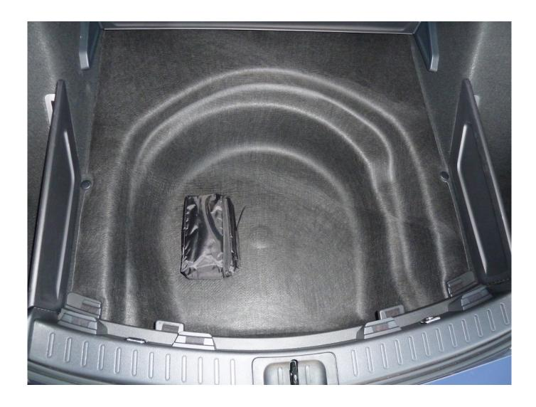
The main boot floor panel, behind the rear seats, can be set at one of two levels, very handy for carrying relatively tall objects. In addition this floor panel can be reversed/turned-over so that the normal carpet-covered face is replaced by an easily wiped clean resin surface – ideal for carrying wet dogs, muddy boots, etc.
