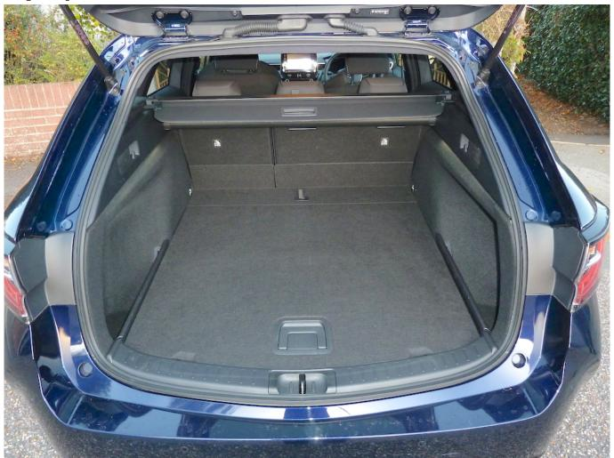
The rear seat backrests – divided two thirds: one third – can easily and quickly be folded/lowered to provide a long and very useful load bay, by activating a simple lever on each side of the car. The floor is not quite flat with the seat backrests folded, for necessarily there is a low 'step' required to accommodate the backrests, when rotated forwards onto the seat bases.
