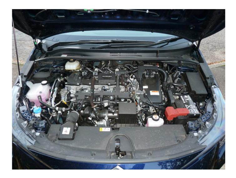
Just one variant is provided, incorporating a 1.8 litre four cylinder 16 valve naturally-aspirated petrol engine, developing 102 PS and 142 Nm (105 lb.ft) torque, allied to an electric motor producing 53 kW and 163 Nm (120 lb.ft) of torque. The combined total power output is 122 PS. The two units are designed to work seamlessly in harmony with each other, and in so doing minimise emissions (103 g/km) and fuel consumption (WLTP Combined figure of 64.2 miles per gallon).
