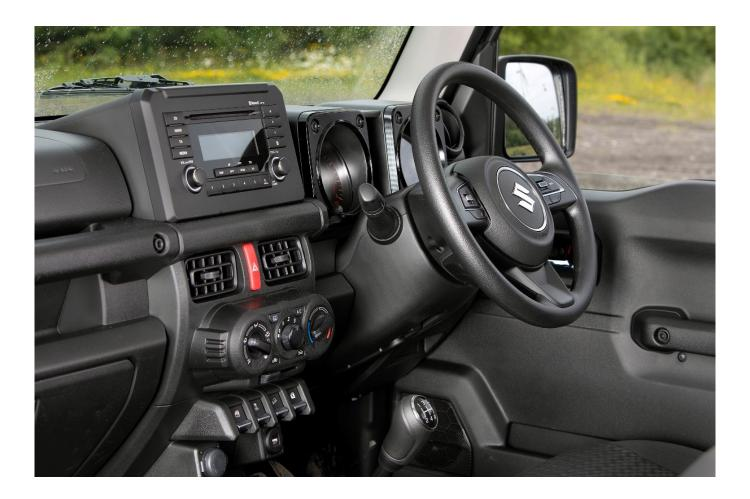
Grab handles for the passenger are useful while the driver hangs onto the wheel, instruments are simple and clear with good straightforward heating and ventilation and powered front windows.
