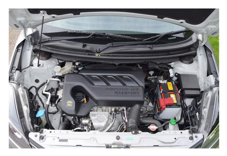
The new three cylinder, direct injection turbocharged (DITC) 1.0 litre Boosterjet motor used in the Baleno produces an impressive 111 bhp, with CO2 emissions of 105 g/km - an SZ5 version of this model, with five speed manual transmission, is the subject of my road test.
