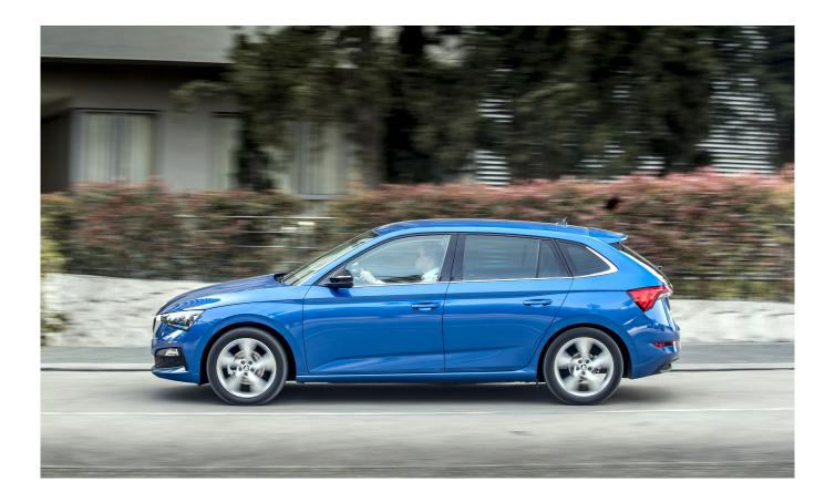
Scala is the first VW Group product to be built on the latest MQB A0 modular platform developed for all future Group models and simply relies on one fixed distance – front bulkhead to front wheels centre-line – and then everything else can be varied to suit. So it produces a changeable wheelbase, track and overhangs.
