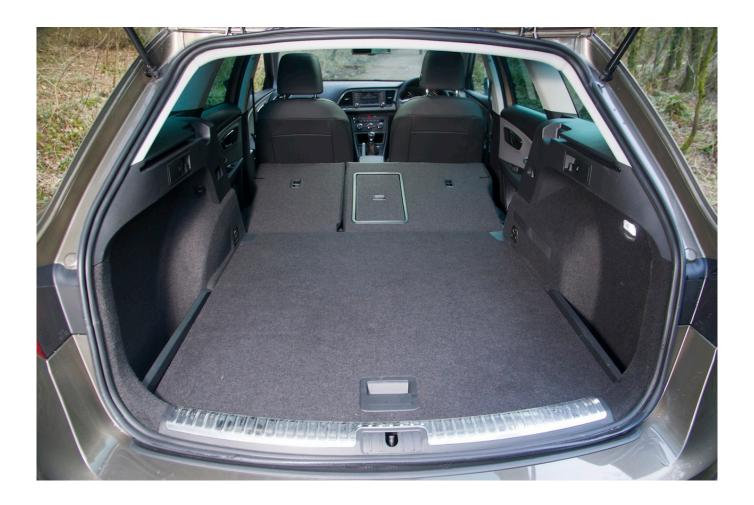
Also, the rear edge of the boot floor curves into the tailgate in a bay shape rather than being squared off to maximise space. Nevertheless, it will take items well over five feet (1.5 metres) long. There is, too, an optional fold-down front passenger seat.
