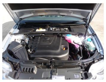
The two litre four cylinder turbo diesel engine develops 143PS; it's a refined and willing unit.
