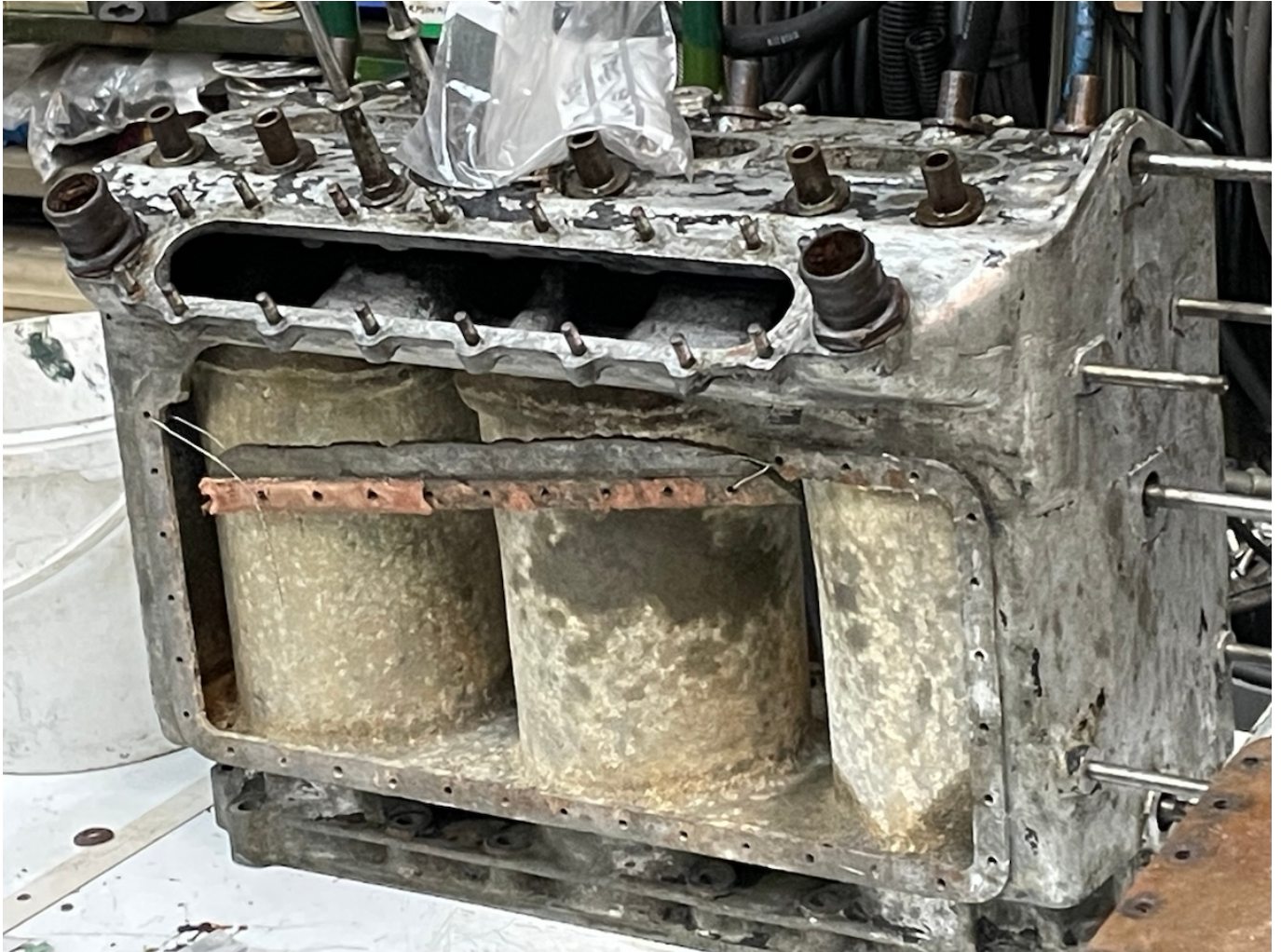
Frost damaged engine block.
