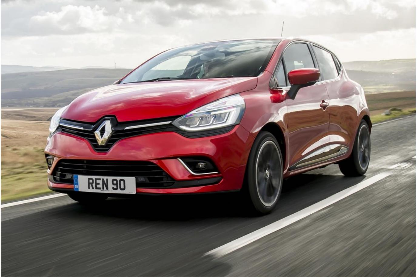
In the 1.2 tonnes Clio five-door body, the 1.5 litre diesel engine pushes out 260 Nm (192 lb.ft) from 1,750 rpm so it pulls very well and showed good flexibility.
