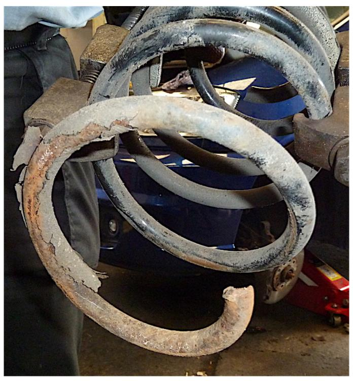
Severe and potentially dangerous mechanical damage to vehicles, such as broken coil springs (like this one) is a direct result of the plethora of potholes in the UK. The problem could become far worse in the near future too...
