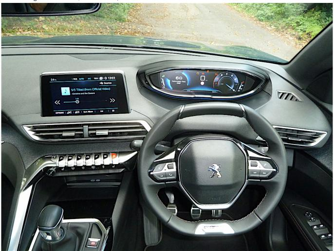
In addition, in the centre of the facia there's an eight inch touch screen, which is visually clear to interpret, and through it the driver or front seat passenger can access the menu controls for a multitude of vehicle systems, including infotainment functions, heating/air conditioning, satellite navigation, 'ambience' settings and so on.
