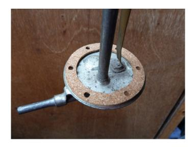
Materials used for fuel system floats and seals in older vehicles (examples shown in the photographs above) were not designed for use with petrol containing ethanol, and can disintegrate if exposed to it; the higher the level of ethanol, the more severe is the problem – and potentially this can cause a serious fire risk..
