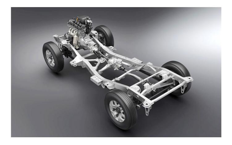
In addition, the engine capacity has been increased to 1.5 litres (from 1.3 litres), delivering greater torque across the rev range, compared with its predecessor. Strong torque output at low engine revs is handy for normal on-road driving but especially useful for serious off-road use.
