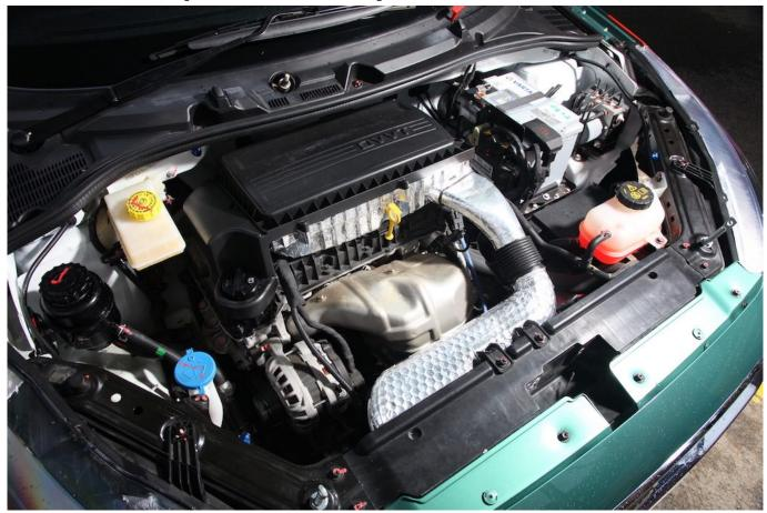
As a result of the weight saving and the use of uprated air filters, the MG3 has gained another five horse power over the standard road car, giving it a recorded 110 bhp which, while still not particularly impressive should be sufficient to ensure some close racing.
