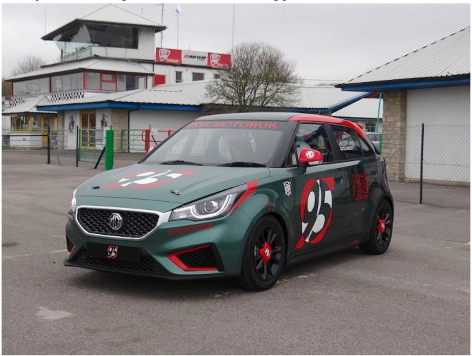
To meet competition regulations the interns stripped out the interior (including the removal of noise insulation and unnecessary brackets) – this took 118 kg off the weight of the car. They then fitted a Scorpion exhaust, K & N air filters, EBC brake pads, Aeroquip steel braided brake lines, installed a full bolt-in roll cage, adjustable race seat, four point harness,
