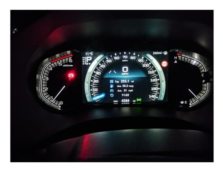
The displays are designed to advise the driver of the operational state of a wealth of vehicle systems (including the Advanced Driver Assist Systems), in addition to showing information such as speed, fuel level, engine temperature, outside/ambient temperature (with ice warning), also covering 'system health checks' and trip computer aspects.
