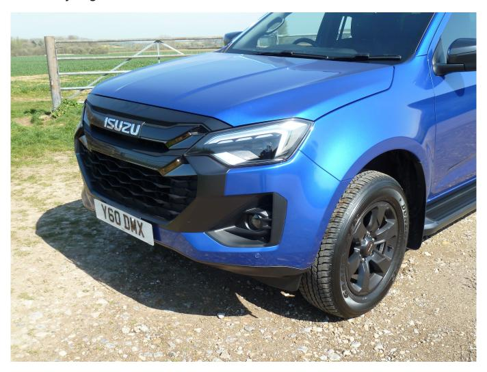
Across the range, the new D-Max models have a noticeably bolder new appearance, including a restyled front grille, new design headlamps (halogen on the Utility and DL20; Bi-LED types, with integrated LED daytime running lights and indicators, on the DL40 and V-Cross).
