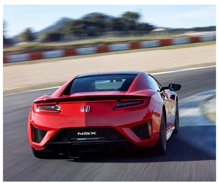
Replacing a planned V10, the 3.5 litre V6 unit develops about 500 bhp, enough you might think, but hang on this is the NSX and it comes with a 47 bhp electric motor/ generator positioned between the engine and the gearbox. Together they work through a nine-speed dual clutch automatic box to send their combined power to the back wheels.
