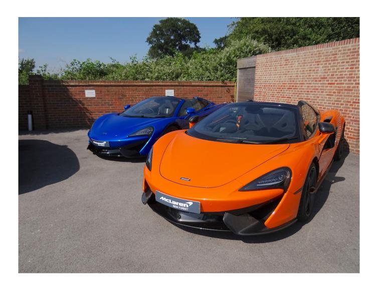
Among McLaren's claims for its sleek and elegant carbon-fibre and aluminium GT are that the new stand-alone model has space for 570 litres or 20.13 cu.ft of luggage (the same as a Ford Focus). Of this 150 litres or 5.30 cu.ft are to be found under the bonnet in a very useful compartment that you can have fitted with McLaren luggage bags.
