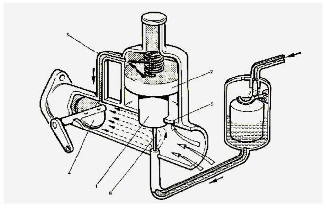
Essentially simple but highly efficient... SU carburettors through the years (and shown is a later example) supplied fuel through a variable jet, to mix with incoming air. More detail on this set-up will follow in Part 2 of this feature.
