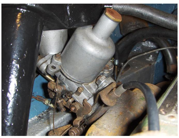
Typical single SU carburettor installation, in this case on an early BMC Mini 850. Similar instruments were fitted to a host of BMC/BL cars.
