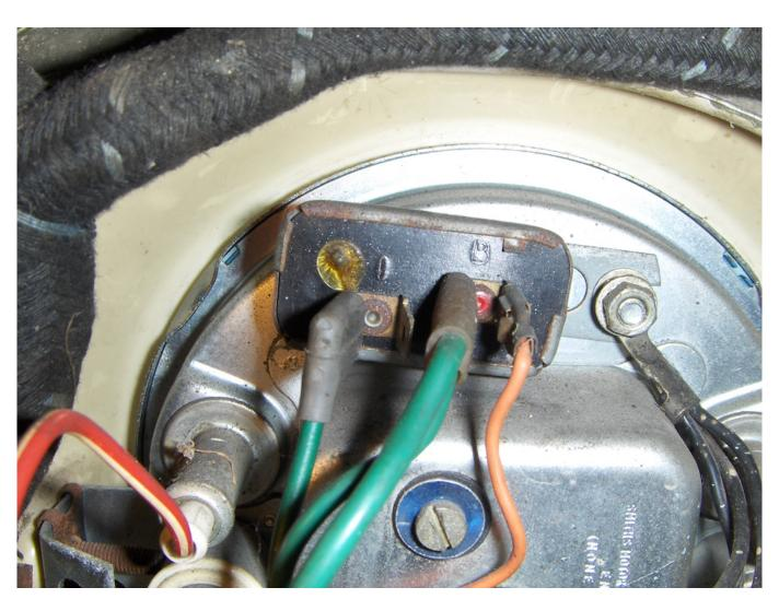
An instrument voltage stabiliser unit in situ in a BMC Mini.
