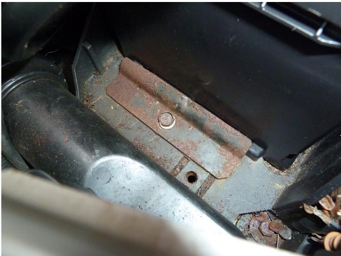
If you have time, remove, clean, de-rust and repaint the clamps/brackets as well. (Yes, that's the next job required on the clamp shown above!).
