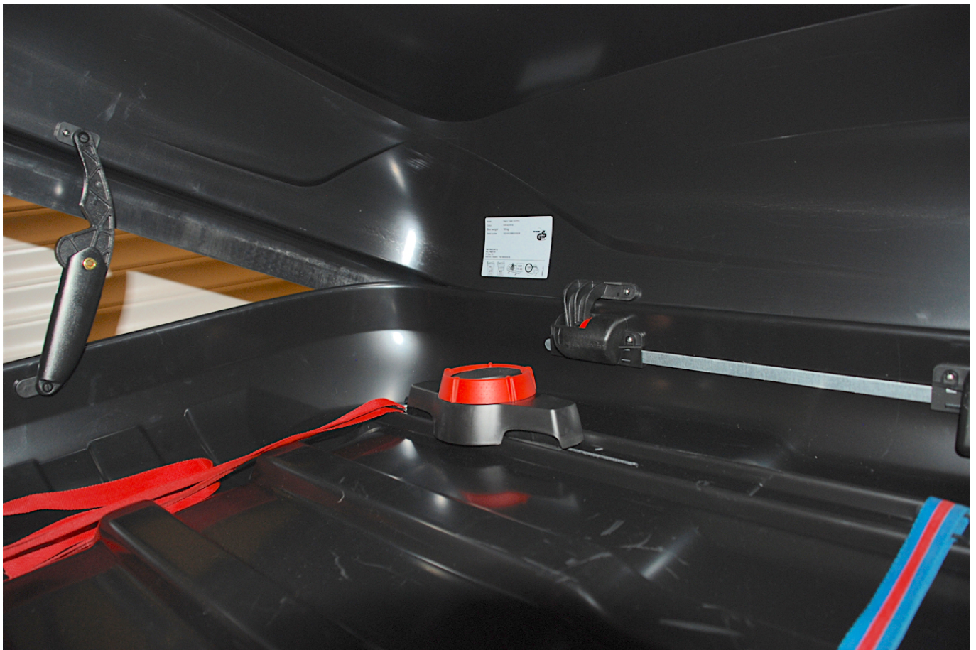
Central hinge at each end, and lock connected to metal bar and straps...
