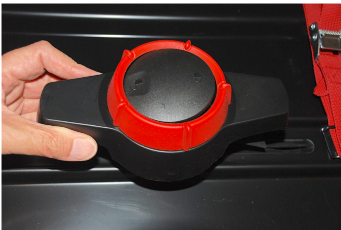
Premier Fit clamp has large adjuster wheel, with 'press down' lock in centre...
