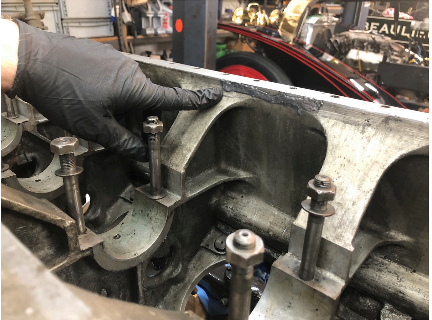
Crack found and repaired with laser welding on crankcase.
