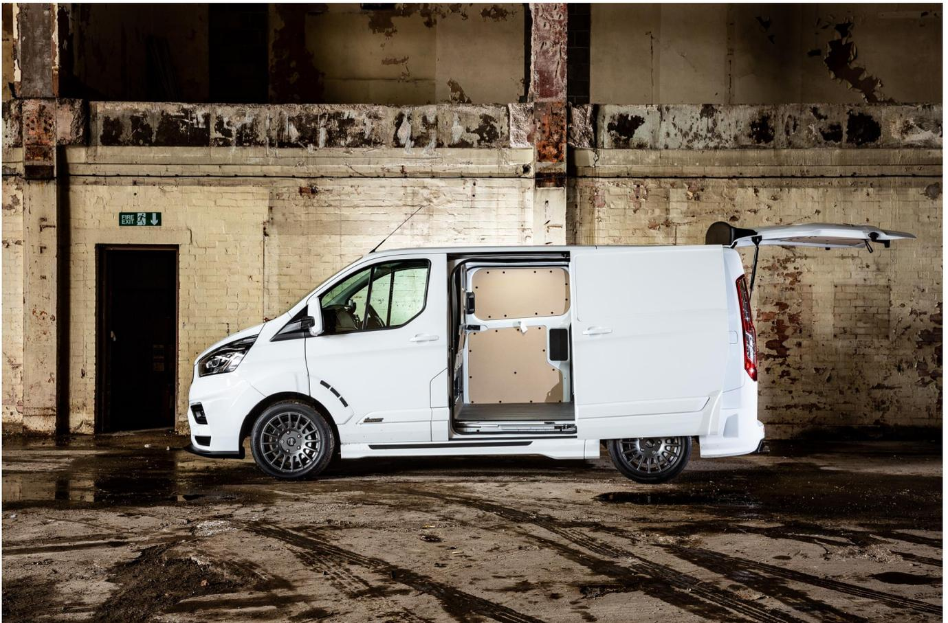
Each van supplied by Ford for the conversion is stripped out, new leather seat covers are fitted in the Welsh factory, a hand-built exhaust is shaped on site, suspension replaced and the bespoke body panels are moulded, trimmed, painted and fitted over about three weeks.
