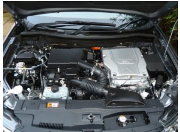
The underbonnet compartment accommodates both the petrol engine and the forward electric motor (there's another one at the rear of the vehicle!).
