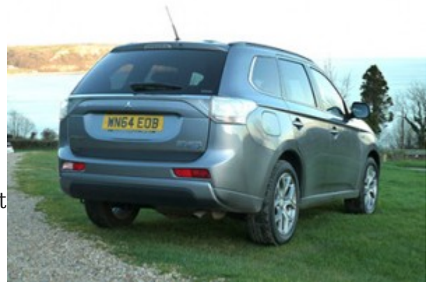
Large, wrap-around, highly visible rear lamp units are excellent from a safety point of view. Note the wide rear doors, aiding entry to and exit from the car.
