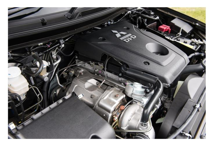
The well-proven 2.4 litre turbodiesel engine is strong thanks to the 430 Nm (317 lb.ft) of torque. It can sound a bit agricultural on start-up but essentially it is a commercial vehicle so it lacks some of the refinement in the powertrain department compared to an SUV.
