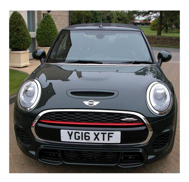
The new Convertible has an overall length of 3,821 mm (12.54 ft) or 3,874mm (12.71 ft) for the Cooper S and JCW versions with their larger sports bumpers. All models are 1,727 mm (5.67 ft) wide, 1,415 mm (4.64 ft) high with a wheelbase of 2,495 mm (8.19 ft). Compared to the outgoing soft-top version there is 98 mm (3.86 in) extra length, 44 mm (1.73 in) extra
