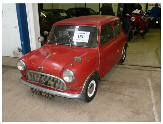
This early Austin version is identifiable by its original 'wavy' grille. (By the way, the 'Flying A' attached to the bonnet of this car is not in fact a Mini feature, but was originally fitted to an Austin A30).
