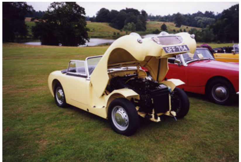
The model from which all later Sprites and Midgets evolved was the Austin Healey 'Frogeye' Sprite, introduced in 1958. The wide-opening bonnet was unusual at the time.
