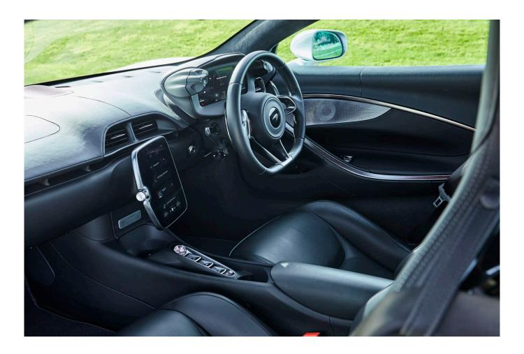
All essential instruments are now contained in a pod fixed to the top of the steering column and displays speed, engine revs. fuel & traction battery state and also carries sequential rocker buttons for power mode and dynamics just a fingertip ahead of the wheel-rim.
