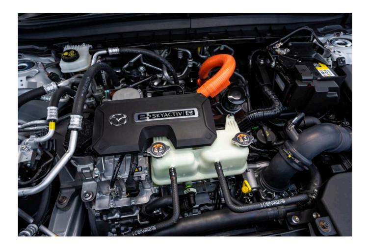
With a 17.8 kW traction battery range of about 53 miles the rotary petrol engine will kick in when needed to deliver a combined range over 400 miles. So you have no real worries about range anxiety as maybe the case in a pure battery electric vehicle.
