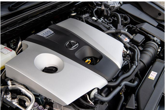
The Lexus ES 300h in the UK has only one power unit option; other countries have the choice of non-hybrid petrol engines. The self-charging petrol-electric hybrid system uses a 2.5 litre, four cylinder 16-valve DOHC petrol unit with dual VVT-i valve timing, mated to an electric motor/generator. Drive to the front wheels is through the usual CVT auto
