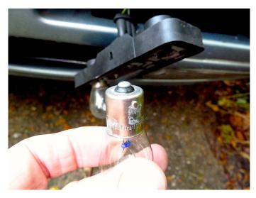
On this Jaguar non-illumination of an indicator bulb was due to minor corrosion on the bulb and its holder.
