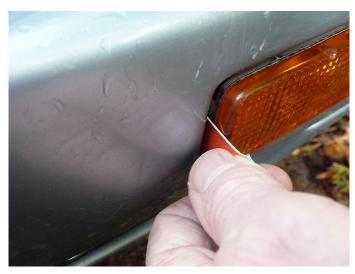
Removal of this lamp unit required a 'special tool' to release its securing clip. I cut a strip from an old plastic card, which...
