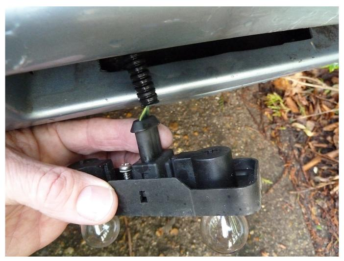
Always treat with care the lamp unit and other components. Ensure that the cables and connectors are clean, sound and firmly attached.
