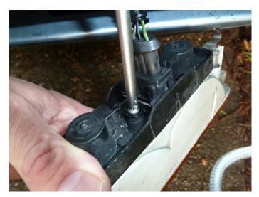
On re-assembly, ensure that all the screws and retaining clips are fully engaged (but don't apply too much force). Lubricate screws to aid installation (and to help prevent seizure in the future).
