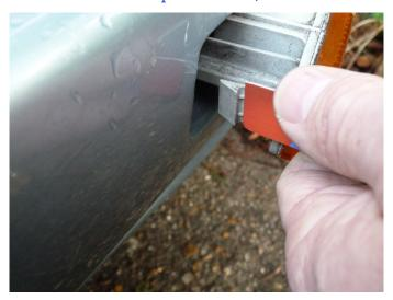
...is gently pushed against the retaining clip like this, to allow the lamp unit to be eased from the bumper.
