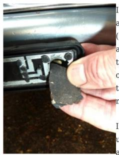
Carefully cleaning up the bulb and its contacts, plus the to that used during dismantling. holder, using a small piece of fine grit abrasive paper, removed the corrosion and restored operation of the bulb.
