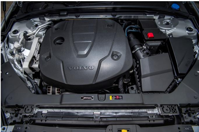
The 2.0 litre D4, four cylinder turbodiesel engine produces a healthy 190 hp with 400 Nm
