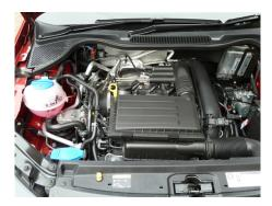
The 1.2 litre petrol-powered Polos have a four cylinder TSI engine (the 1.0 litre cars each feature a three cylinder motor).
