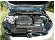
Under the bonnet of the 1.6 litre TDI as test-driven is a 110 PS version of VW's refined and economical four cylinder turbo diesel engine.
