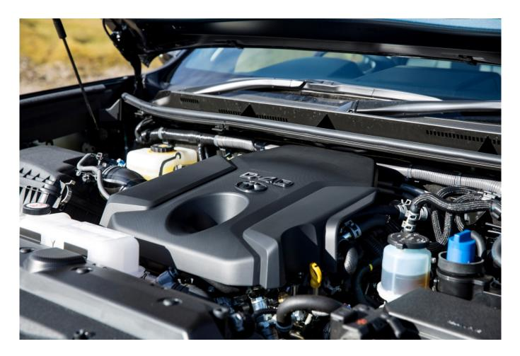
Official combined cycle fuel consumption is 38.1 mpg with 194 g/km CO2 emissions. The engine is also available in the Utility version with a six-speed manual gearbox where the maximum torque of 420 Nm (310 lb.ft) is available from 1,400 to 2,600 rpm. Acceleration to 62 mph takes 12.0 seconds, while the benchmark figures for fuel economy and CO2
