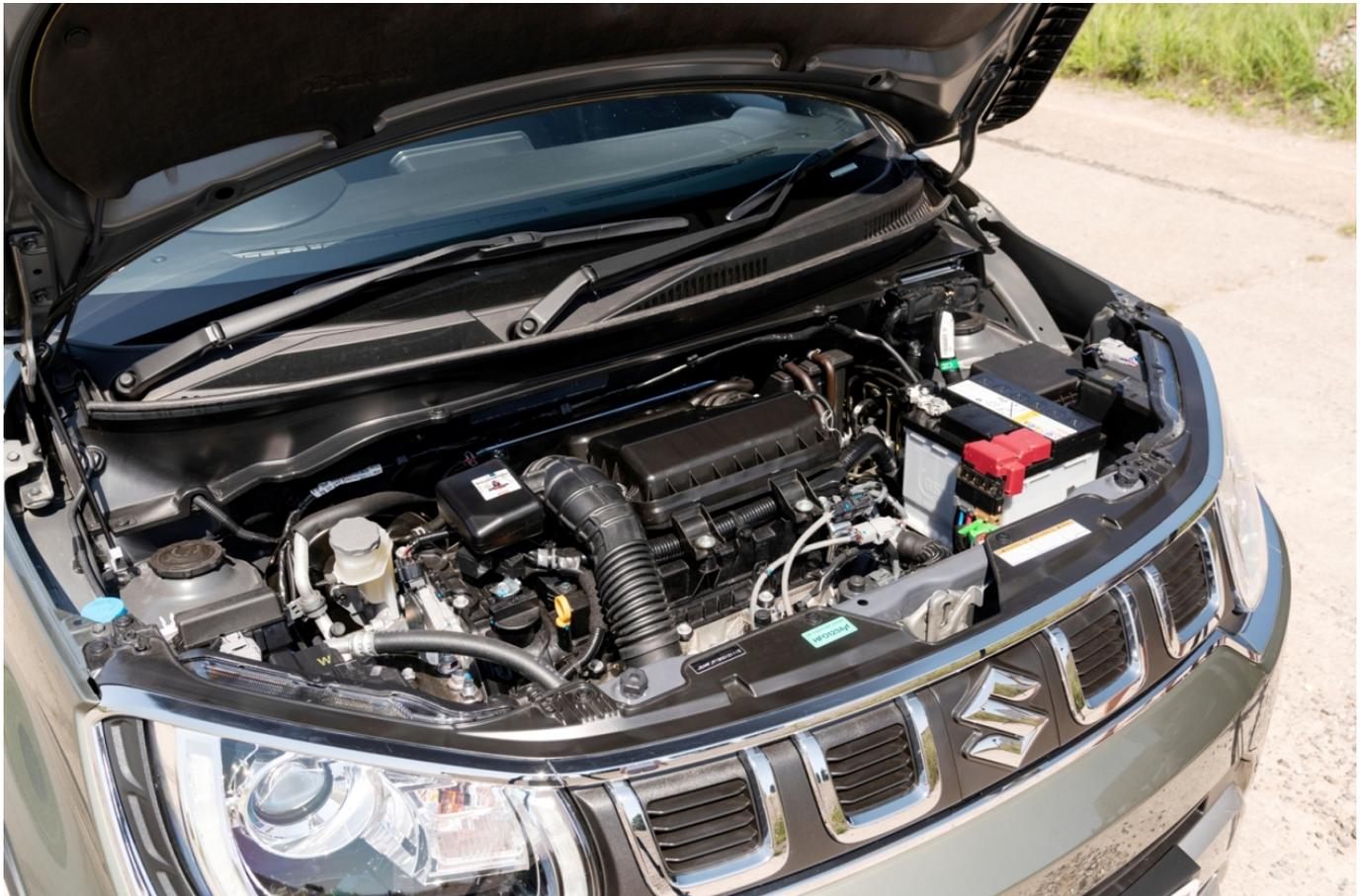
The engine is paired with a 12-volt self-charging hybrid system and new 10 Ah lithium-ion battery. The hybrid system uses an Integrated Starter Generator (ISG). This unit is belt driven and assists the petrol engine during initial vehicle take-off and acceleration modes. It also generates electricity through regenerative braking recharging both the lithium-ion battery and the conventional 12-volt battery and it operates the fuel saving Stop/Start system.
