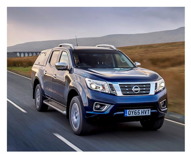
The Double Cab versions, the choice of 95% of UK Navara customers, uses a heavy duty ladder frame chassis but this time with a multi-link style rear suspension with coil springs rather than the widely used leaf spring layout of its competitors. This gives a more
