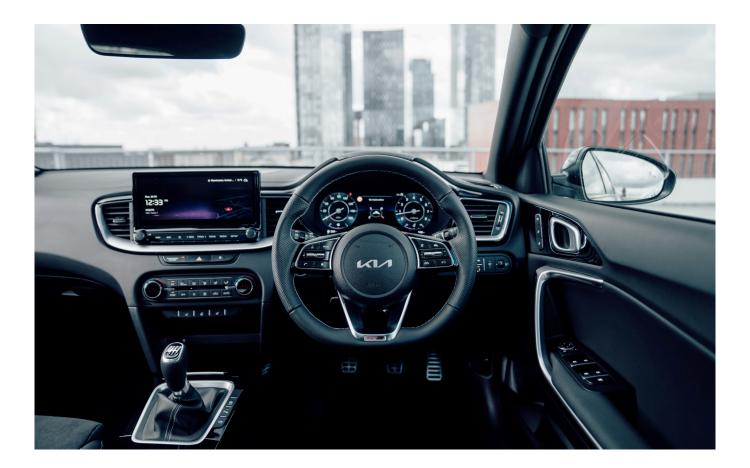
KIA has simplified the touch-screen without losing its effectiveness and clarity and now fitted sensitive touch buttons for the audio volume, heating and ventilation on the lower fascia where most likely to be used by driver or passenger. It's a wise move and less distracting than used through a screen.
