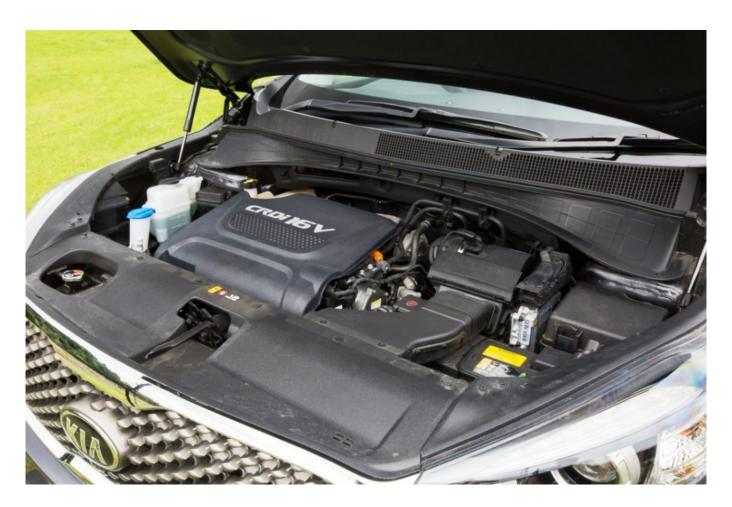
The revised 2.2 litre, four cylinder turbodiesel engine with 197 bhp and 441 Nm (325 lb.ft) of torque available from 1,750 rpm is a strong and responsive unit and its sounds relatively refined. It works well with the smooth changing eight-speed automatic gearbox. The down-changes are not as quick as some twin-clutch units but for most users that isn't an issue, it's refinement that counts. The various driving mode settings are useful as well.
