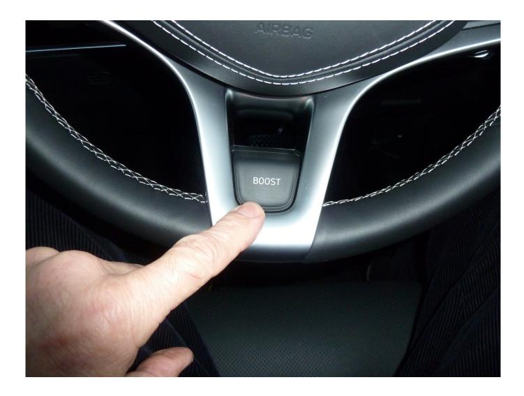
To show the difference, acceleration from rest to 62 mph is quoted at 4.8 seconds (itself an impressive figure) when driving normally, by this is reduced to 4.2 seconds by using the Boost facility.
